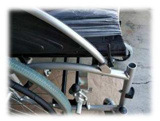
At the point where the armrest meets the seat, there is a reset lever. Push it back and push the armrest down to lock it. Release the lever to return to snap the hole.
