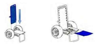
8. To mount the arms left and right follow the image below and tighten the screws to ensure their stability.
