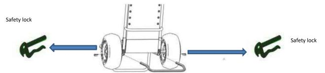
6. To replace the front wheel, remove the safety locks that are present - lock the wheel and replace the new wheel you want by locking it again with the safety locks you previously removed as shown in the photo below:
