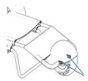
7. To remove the back and seat fabric, remove the safety locks and pull the fabrics out. Just by following the same procedure you can replace the fabrics. Check out the following photos:
