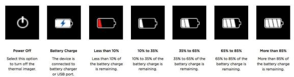
**NOTE:** This device will provide up to 3.5 hours of imaging time with a full charge.
