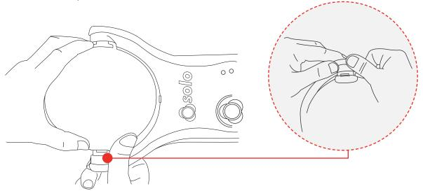
Fit the ASD adaptor by locating into both arms. Ensure that the fan symbol is located on the side of the unit where smoke is emitted. (LHS when unit is facing the user).
