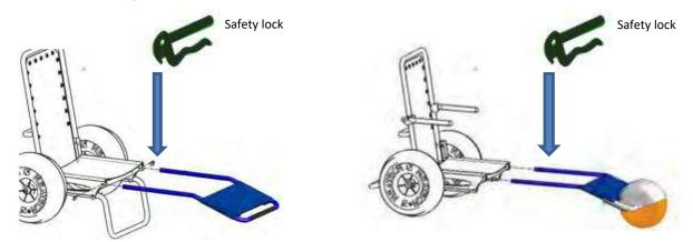
5. If you want to remove the anti-tilt section, remove the safety locks and then remove the extra section as shown in the photo below:
